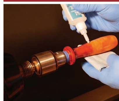
You can apply GluBoost's Fill n' Finish to small turnings as a finish while they are still on the lathe.
