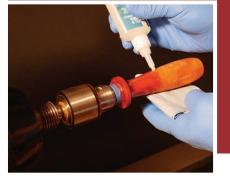
You can apply GluBoost's Fill n' Finish to small turnings as a finish while they are still on the lathe
